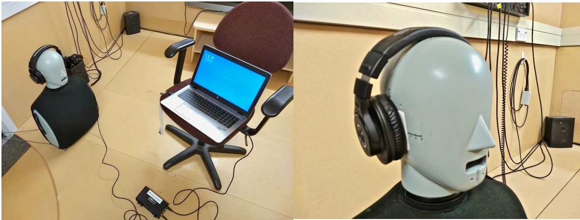
Figure 3.2 The same Brüel & Kjær model 4100 head and torso simulator used for calibration in EXP.1 is shown 'wearing' the Audio-technica ATH40x headphones used by all participants in this study. On the left we see the experimental setup as participant would later experience it; on the right we see a close-up of the ATH40x headphones during calibration.
