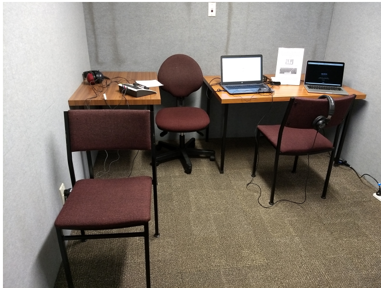
Figure 3.1 The experimental equipment as it was set up for each session in the sound attenuated booth. From bottom left in clockwise fashion: A chair for participants to face away from the experimenter during the hearing screening; the hearing screening station with headphone and the Interacoustics AS608 audiometer on a table; a chair for the experimenter during the screening; the HP Elitebook running the experiment; the USBPre audio interface; a sign instructing participants how to navigate the two experimental platforms; the Macbook Pro running 'Quinn'; a chair for the participants during the experiment; and the ATH40x headphones resting on the chairback.
